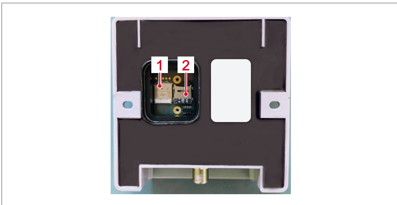
Fig. 10: Slots – SIM card and microSD card
